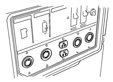
To stop the engine in an emergency, turn the engine switch OFF.
